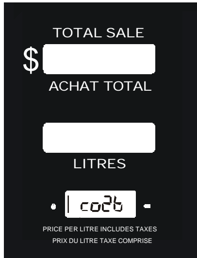
FIGURE 7 – FAULT CODE DISPLAYED BY MICON 550LN ELECTRONIC REGISTER
